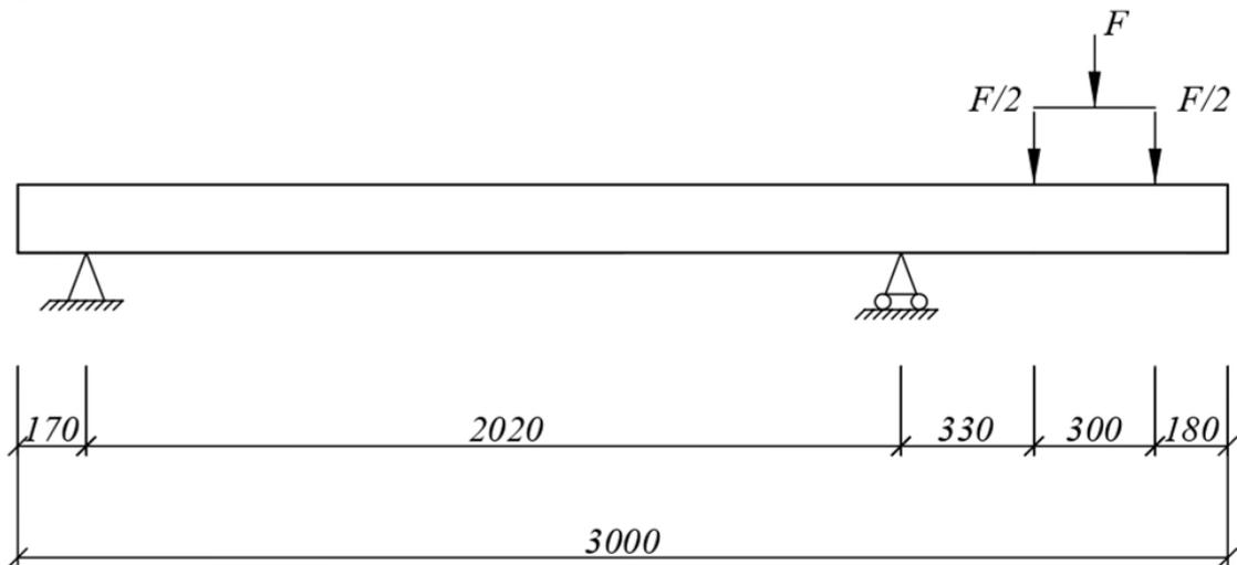
Fig. 2. Cantilever loading scheme
