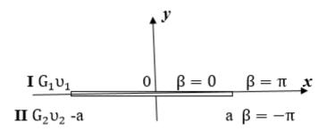
Fig. 1. Composite plane with a finite crack
