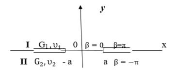
Fig. 2. Composite plane with an infinite crack
