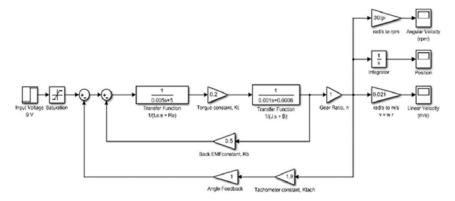
Fig. 2. Motor implementation on Simulink
